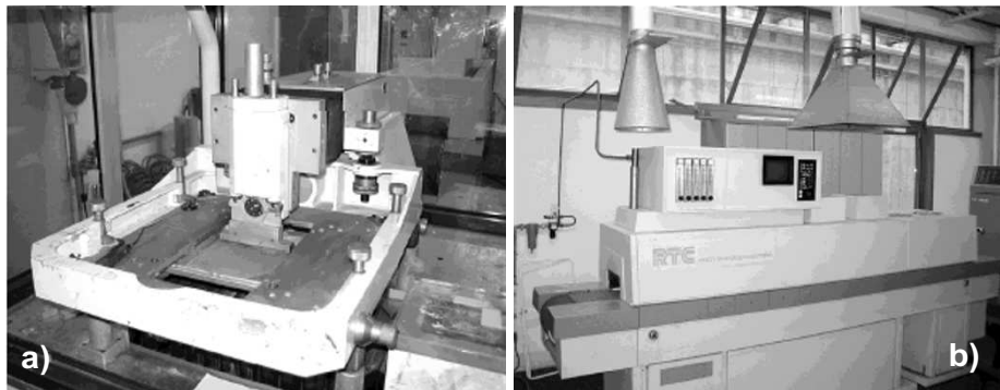
Figure 2. Screen-printing Machine (a) – Infra-red Belt Furnace (b).
